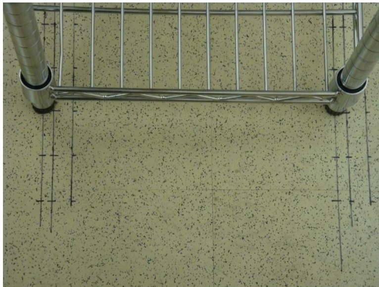
Figure 9: Graduation marks for varying distances during laser calibration
