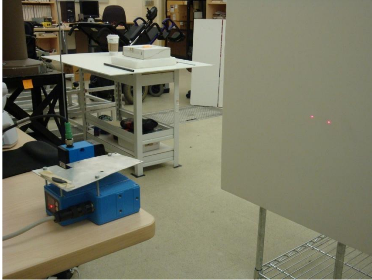
Figure 8: Laser calibration set-up
